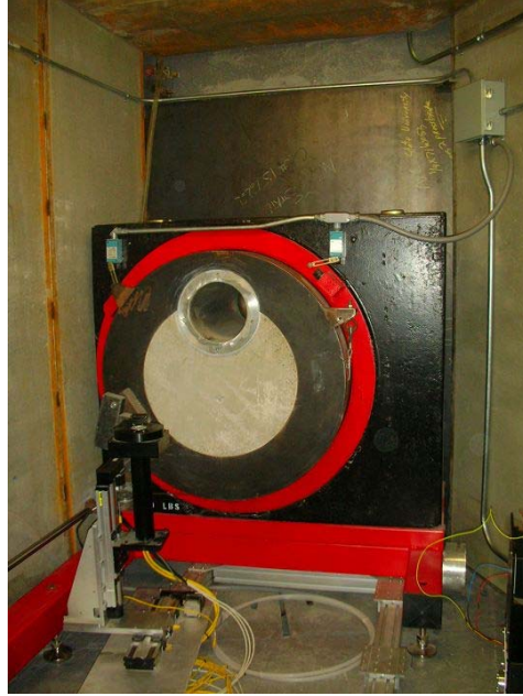
Figure 3.15: Close-up of the thermal neutron beam port.
