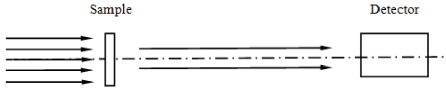
Figure 2.9: Principle of a transmission experiment.
